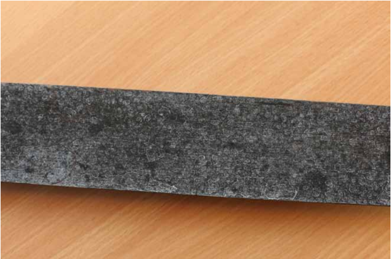
fig.17 : wood coated with fungus to increase its resistance to environmental factors and its durability
