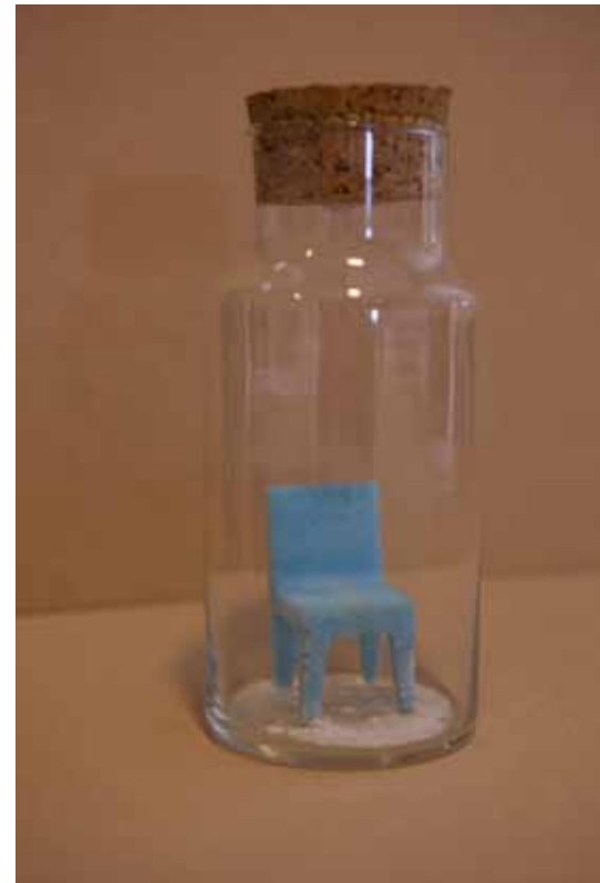
fig.14 : Phanerochaete Chrysosporium: experiment on plastic chip and polystyrene model
